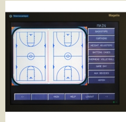
TSC2000XL Advanced Electronic Control System and Touch Screen
