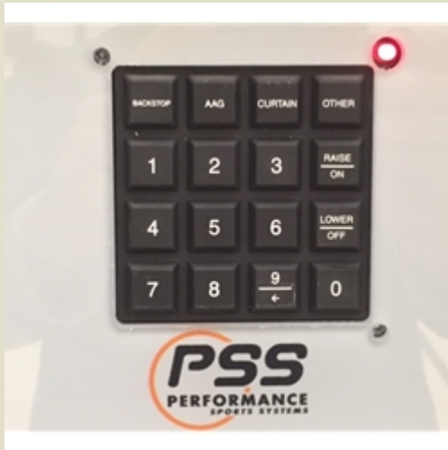
TSC1500 Electronic Control System and Keypad
